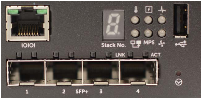
Figure 1-3. Dell Networking N1524P Close-up
